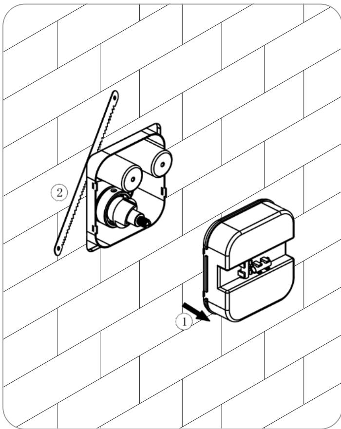
**7.** Remove the box cover and use a saw to cut the raised part. After cutting, make sure the plastic does not protrude above the wall.
