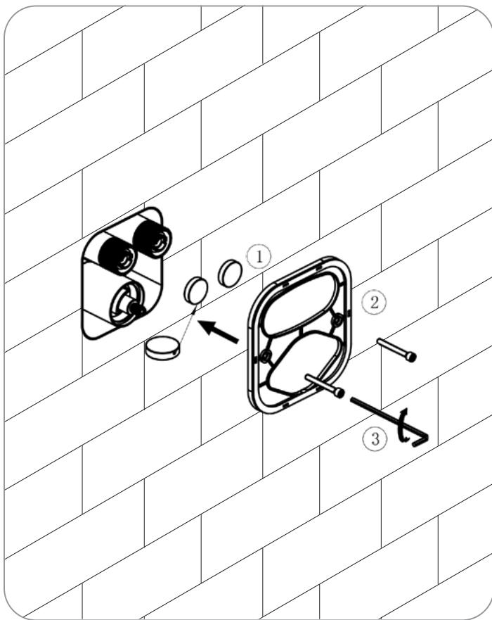
**9.** Install the button guards and the sealing plate according to the drawing.
