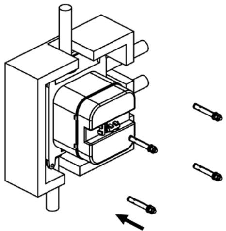
**5.** Fasten the box to the wall with screws and tighten the screws, ensuring that the box is parallel to the wall; monitor the box level and make sure that the box is installed horizontally.
