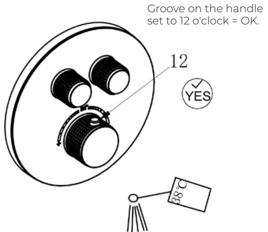
Turn the thermostatic holder and use a thermometer to check the water outlet temperature; if it is up to 38°C, the handle button should indicate 38°C.
