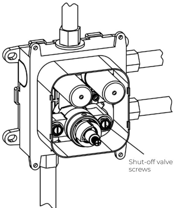
**4.** Use a screwdriver to turn the screws clockwise to close the shut-off valves, which will interrupt the hot and cold water supply flow.
