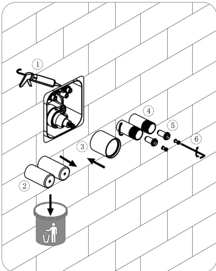
**8.** Remove the protective cover and install the valve parts according to the drawing.
