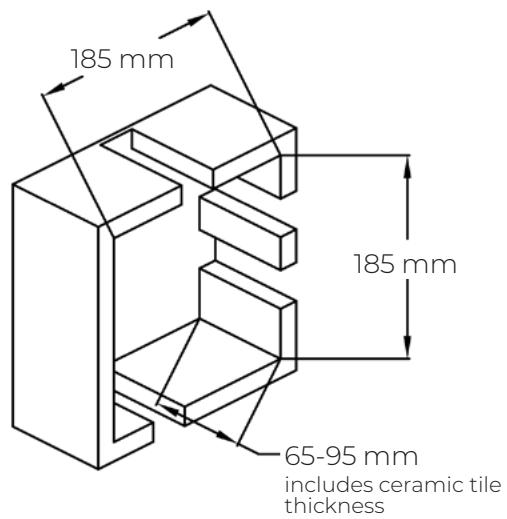
1. Make a cavity in the wall with the size as shown in the drawing.
