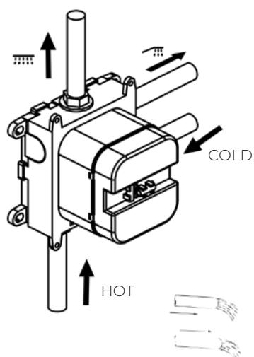
2. Connect hot and cold water supply according to the markings on the body (red – hot water, blue – cold water). Connect the supply to the hand-held shower spray and rain shower head according to the drawing and the markings.
