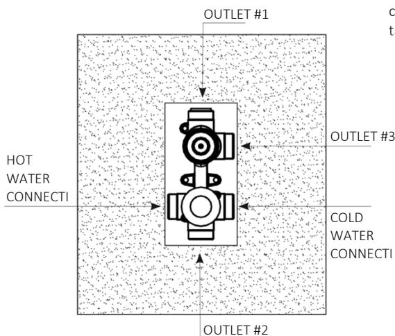
Connect hot and cold water connections to the concealed mixer tap body.
