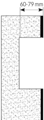
Create a recess in the wall as shown in the figure below.
