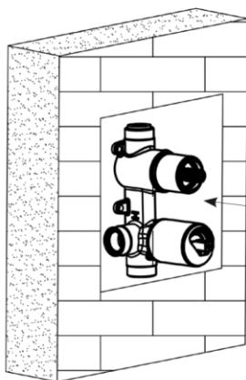
Place the mixer tap rosette (cover plate) on the valves as shown in the figure.
