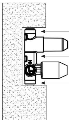
Perform a leak test of the concealed valve to ensure there are no leaks at each installation connection. If the valve and connections are tight, fill empty spaces with mounting foam.
