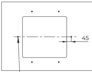
Hole size: Ø10 mm, depth: 15 mm
