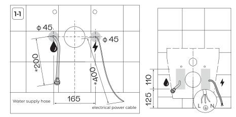
To provide additional protection, it is recommended to install a residual current device (RCD) in the power circuit, with a rated operating current not exceeding 30 mA.
