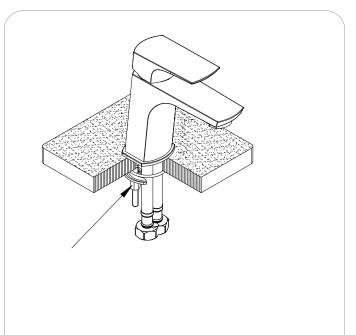
**5.** Ensure that the lock nut is fixed and the tap is stable.
