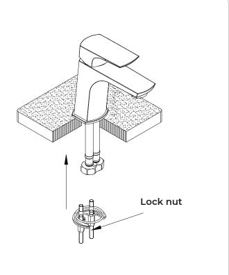
**4.** Place and fix the lock nut under the body of the tap.
