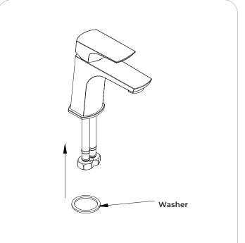
**2.** Install the washer under the body of the tap.
