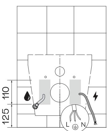
For additional protection, it is recommended that a residual current device (RCD) with a rated operating current not exceeding 30 mA be installed in the power supply circuit.
